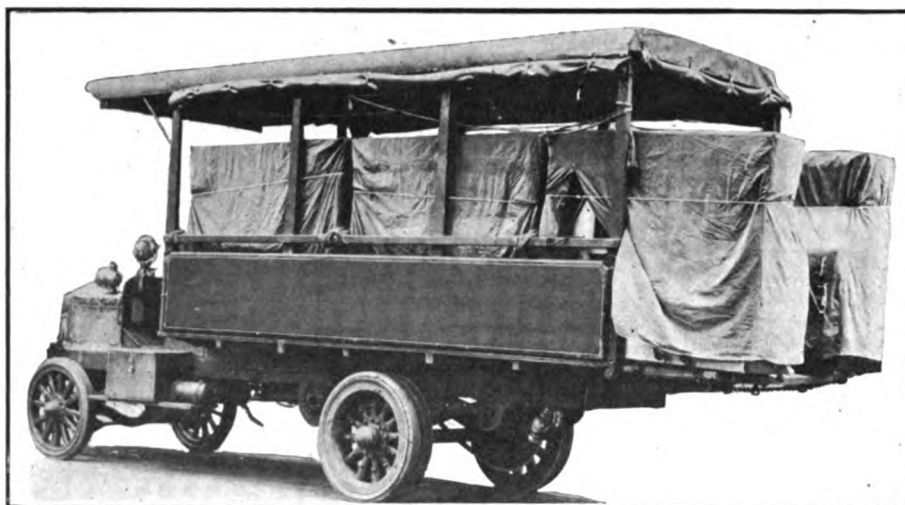
Fig. 3.—Packard 3-ton truck with full load of pianos. Note that the middle pair stand only a trifle in front of the rear axle and that the end pair and forward pair balance each other in such a way as to throw almost 90 per cent. of the load weight on the rear wheels
